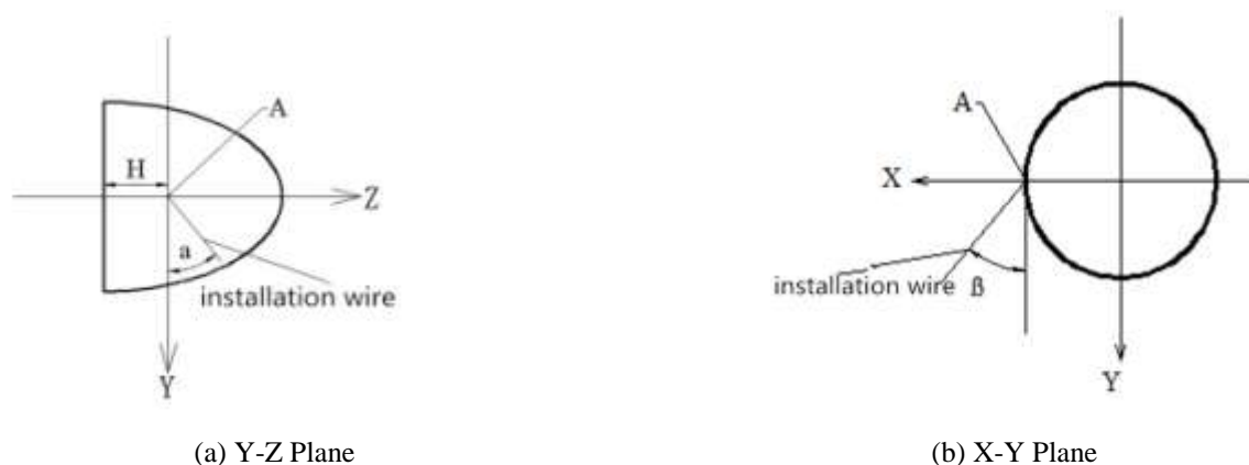
Fig.4 The installation coordinate system of the reamer
